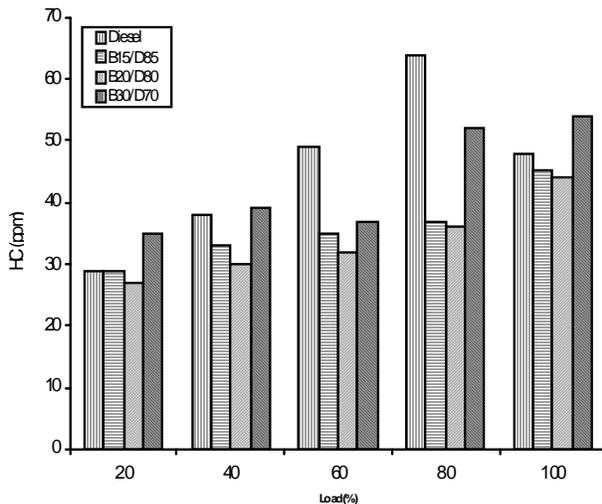
Fig. 6. Hydrocarbon emission Vs load.
