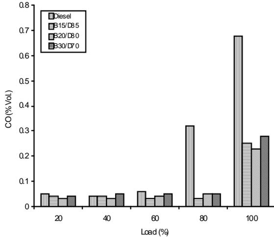
Fig. 5. Co emission Vs load.
