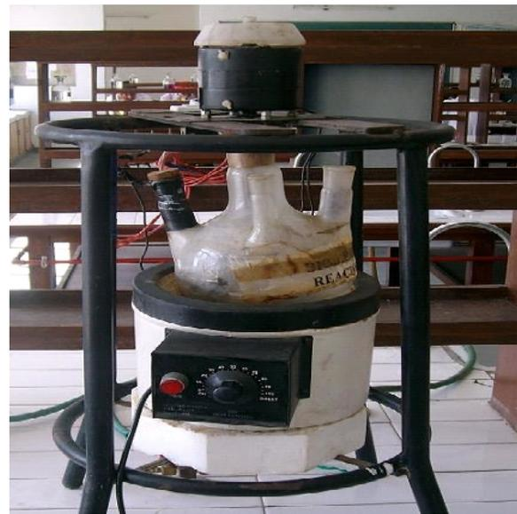
Fig. 1. Biodiesel reactor 2L capacity.
