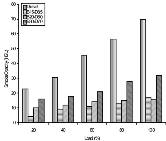
Fig. 7. Smoke opacity emission Vs load.
